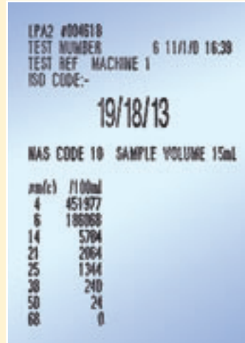
1 Online-normal Single test result. ISO 4406 code.
