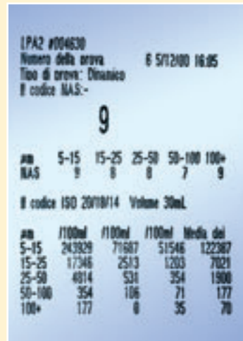
2 Online-dynamic Three test & result average. NAS 1638 code.
