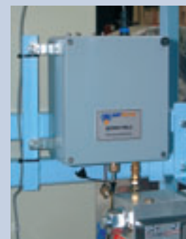
PML2 In-line Particle Counter
