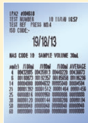
3 Online-dynamic Three Test & Result Average. ISO 4406 code.
