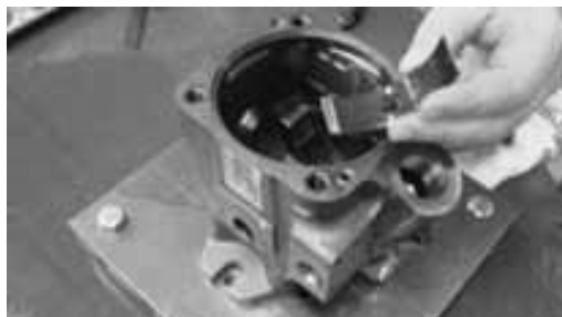
24. Remove Shaft Seal With the seal retaining ring removed use a punch or similar tool to knock out the shaft seal.
